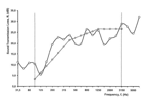
According to the results obtained in the frequency range of 100 Hz to 3150 Hz in 1/3 octave band based on ISO 717-1 standard, calculated weighted sound reduction index
